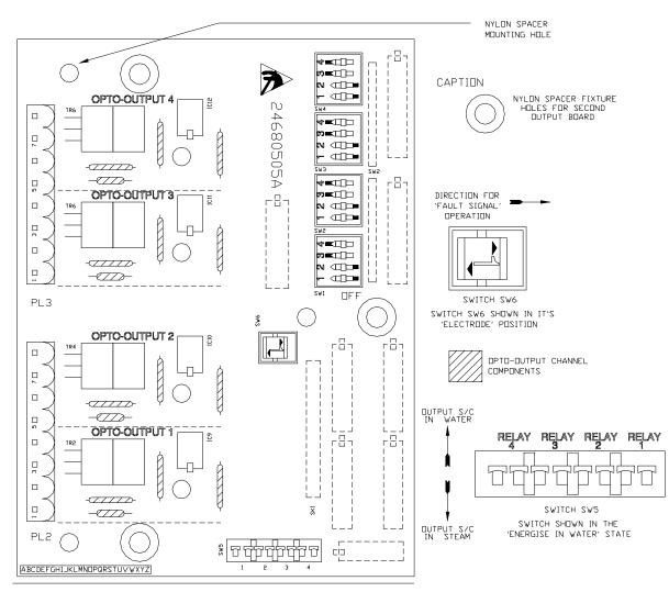
Figure 3c.1 - View of opto-isolated board showing switch positions and output pin details
